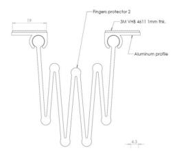
FLEXSAFE $^{\text{TM}}$  V3 — For use on outer frame side (hinges side).
