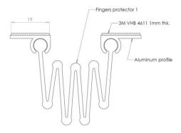
$FLEXSAFE^{\text{\tiny{TM}}}\ V2-\text{For use on extra thick doors, protects from inner frame side}.$
